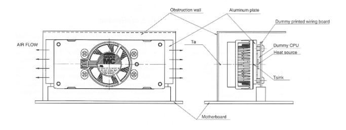
Fig.4 Air flow of an ordinary heat sink fan
